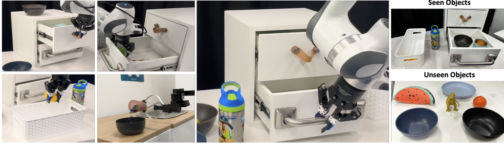
Figure 6: Examples of tasks executed on a Franka arm through our trained model in a clean setting. We trained numerous tasks (left) and tested on both seen and unseen objects (right).
